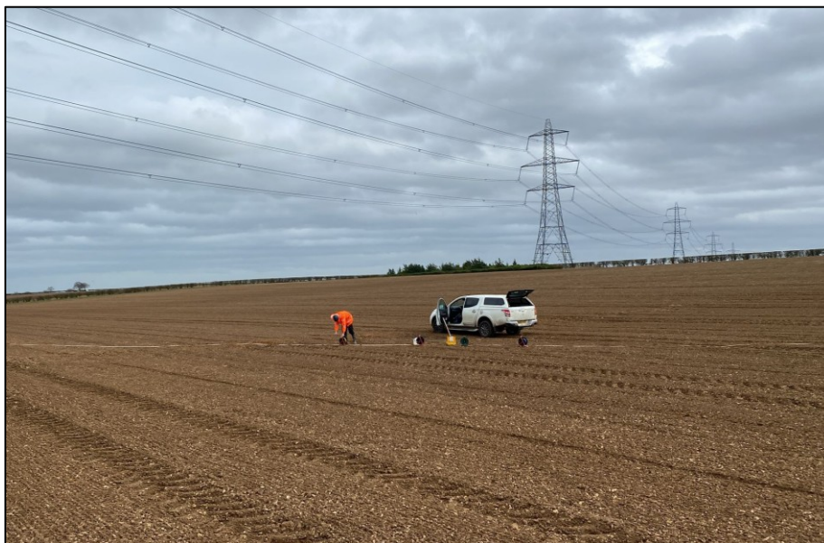
Plate 3 Soil resistivity testing in progress at SR3
