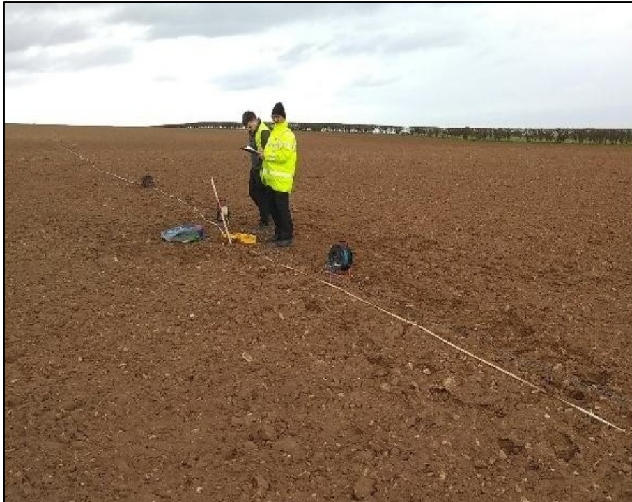
Plate 2 Soil resistivity testing in progress at SR2
